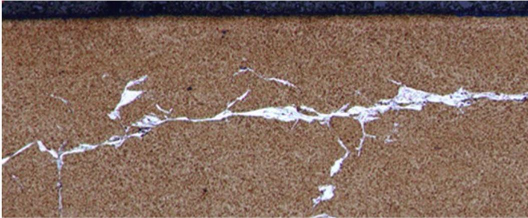
WECs can lead to **premature failure** at e.g. 1% -20% of calculated rating life.
